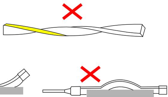
Install and remove with MAX 15° bending, to avoid damages to the circuit
