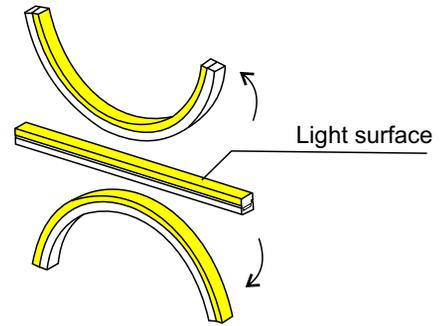
Do not bend more the strip horizontally, this will damage the circuit inside and cause failure
