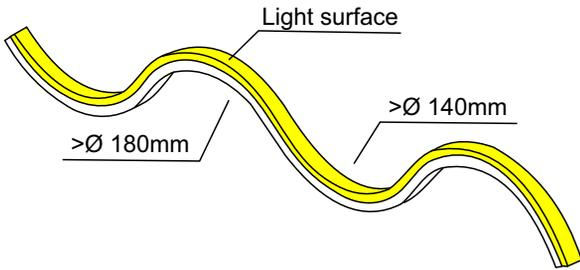
The NEON strip can only be bent laterally
