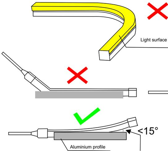
Do not twist the NEON strip, the inside circuit will be damaged and cause failure
