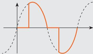
a) Leading-edge phase control: a freely definable portion of the ac voltage reaches the ECG.
