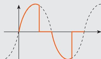
b) Trailing-edge phase control: a freely definable portion of the ac voltage reaches the ECG after passing through the zero crossing point.
